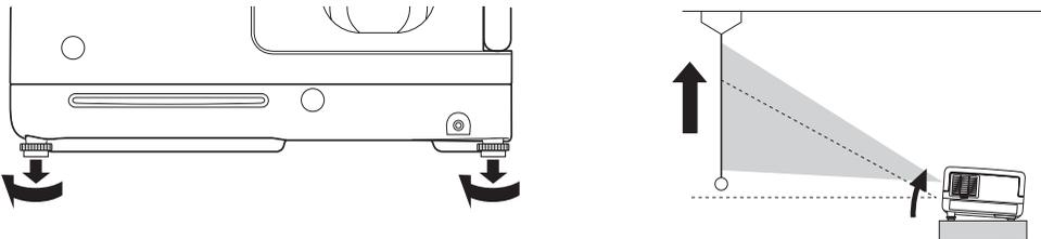
If you tilt the image, it will lose its rectangular shape. Use the **Keystone** buttons on the remote control or the control panel to adjust the image shape.
